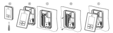
Do not use the supplied screws to mount the unit to an electric box or an equivalent device. The supplied screws are only suitable for mounting the unit to the wall. Ensure to use the appropriate screws for any other application. Tighten by hand only and ensure not to overtighten the screws.
